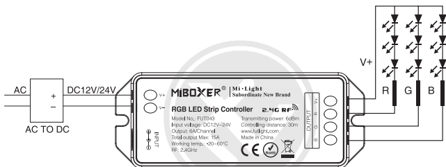
Controller connect to RGB LED strip diagram
